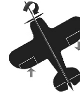
Figure 2 Gyroscope fixed wing turn-right adjustment
